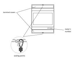
The meter has sealable input and output terminal covers to prevent any attempts to bypass the meter.
